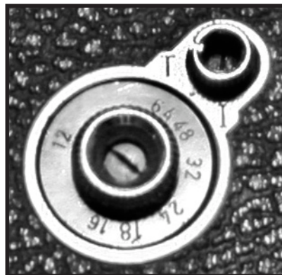
Frame speed select dial and Instantaneous and Time Release selector.
