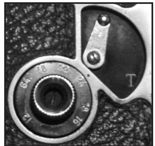
Frame speed select dial and Instantaneous and Time Release selector.
