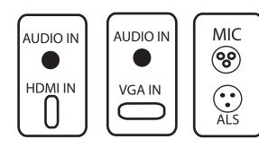
Note: If you are switching between the VGA input and the HDMI input there will be a 10 second delay before your image appears.
