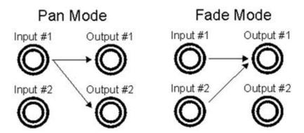
In Pan mode, the control input controls which output input I is routed to.
